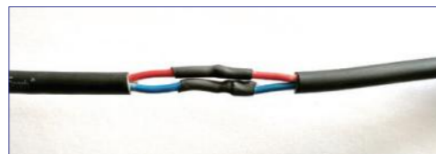
2. Seal the cable with the shrinkable tube.
